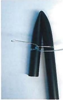
a) Smooth hose closed with tie wire (for PL1 only)
