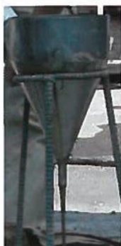
b) US Army Corps of Engineers / FIP flow cone
