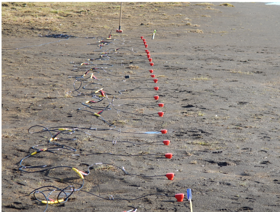
Figure A.3: MASW measurement profile at a test site near Arnarbæli in South Iceland. Lineup of 24 geophones with equal spacing of 1.0 m connected to a seismic cable.
