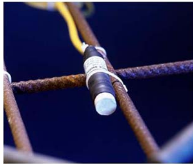
The ERE 20 attached to the reinforcement
