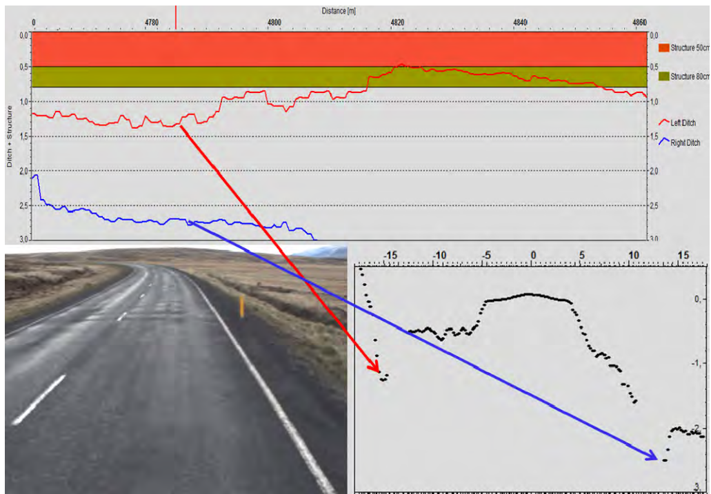
Figure 62: Ditch depth shown as a continuous ditch depth field and as a cross section view at chainage 4785m. The red arrow indicates the left ditch and the blue arrow indicates the right ditch. On the left from 4820m to 4850m there was a short section where the ditch was shallow.
