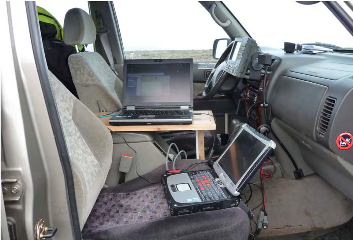
Figure 4: A Toughbook laptop (front) was used for drainage analysis. Red pieces of tape helped to choose the right keys during the survey. A second laptop (back) was used to collect the laser scanner data.
