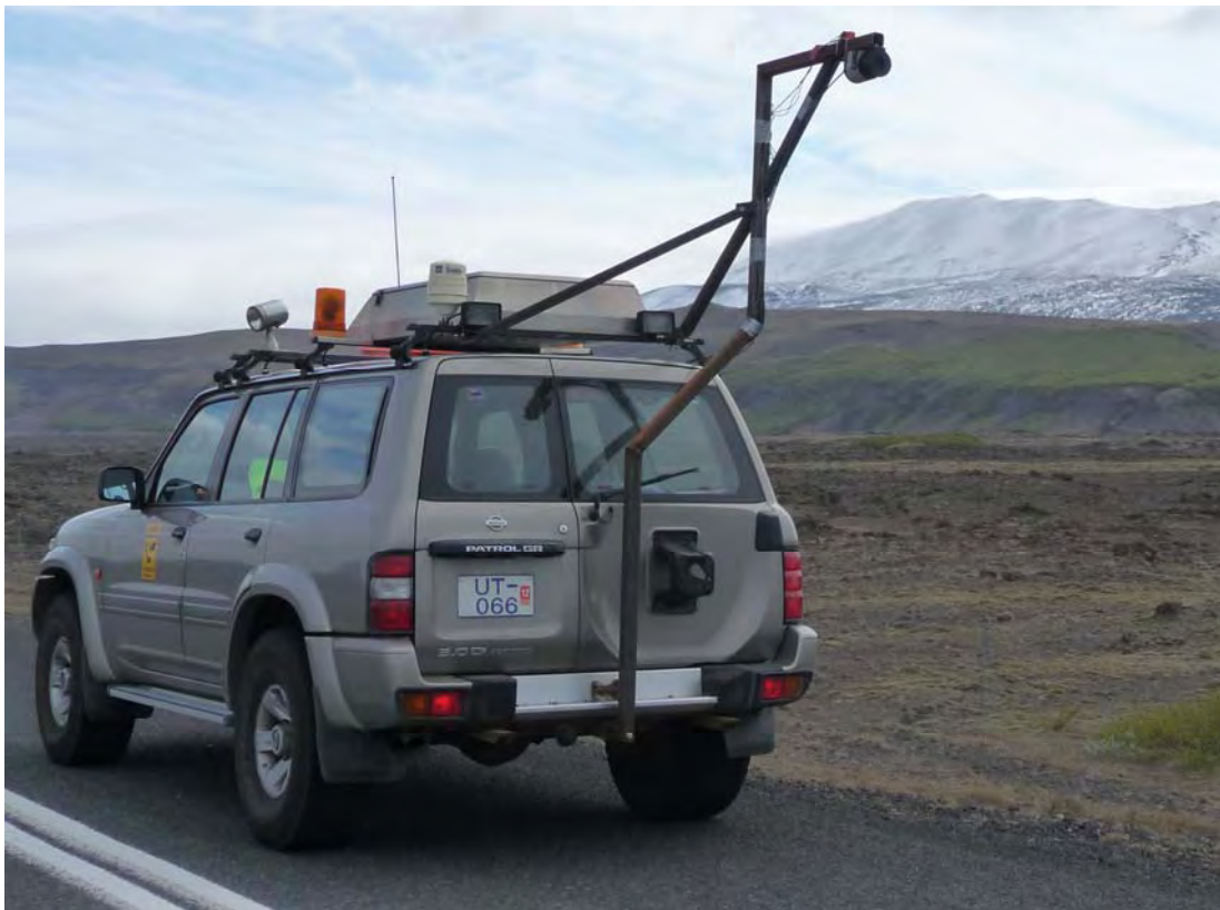
Figure 5: The laser scanner behind the survey vehicle at the height of 3m.
