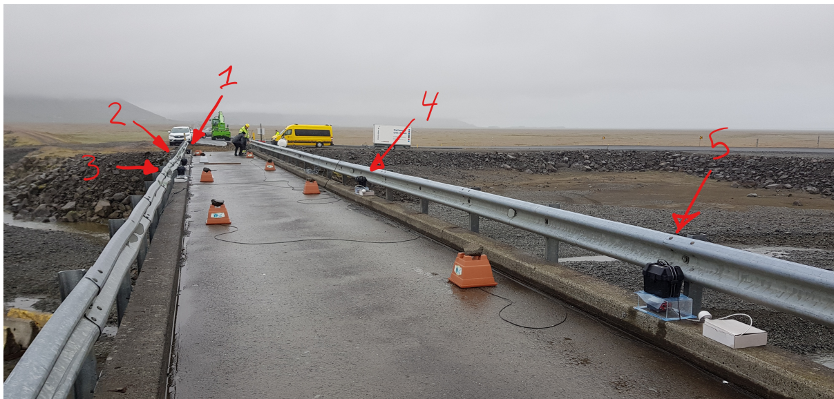
Figure 2.3: Position of the accelerometers in July.
