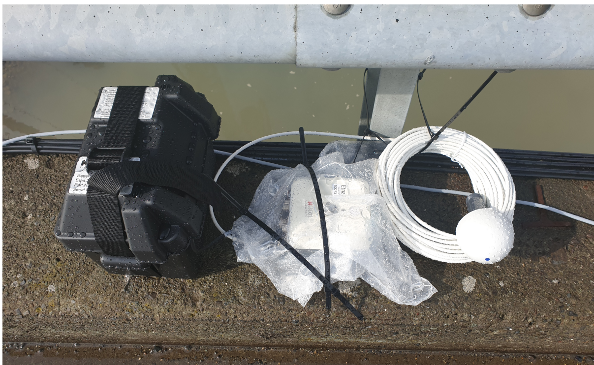
Figure 2.4: Setup of the 3D accelerometers (from left: battery, accelerometer and gps).
