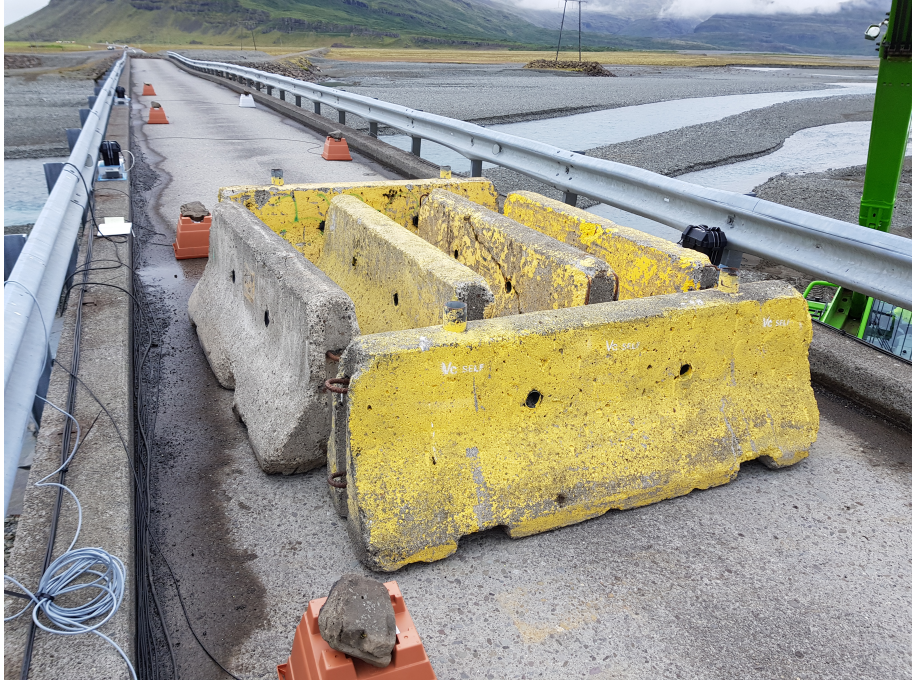
Figure 2.7: The concrete blocks on the bridge span during static testing.
