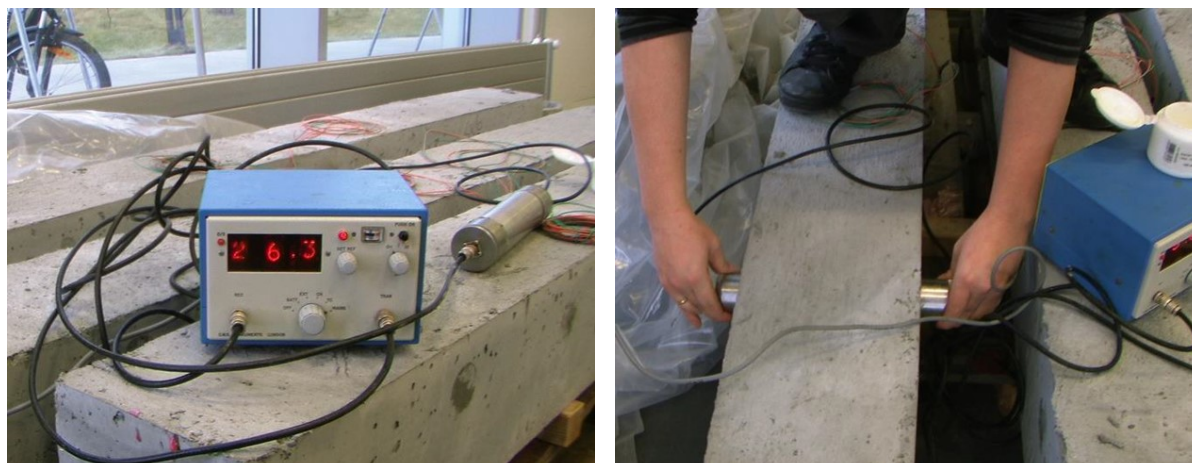
Figure 2.9: An example of the Pundit instrument in use.
