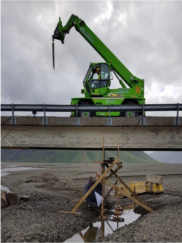
Figure 2.8: The Roto Merlo truck on the bridge span during static testing.
