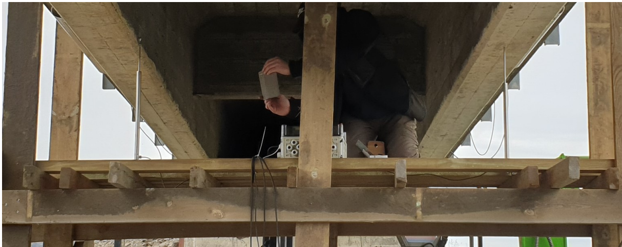
Figure 2.5: LVDT sensors below the bridge deck (left: rod end bearing, right: spring loaded with a ball end).
