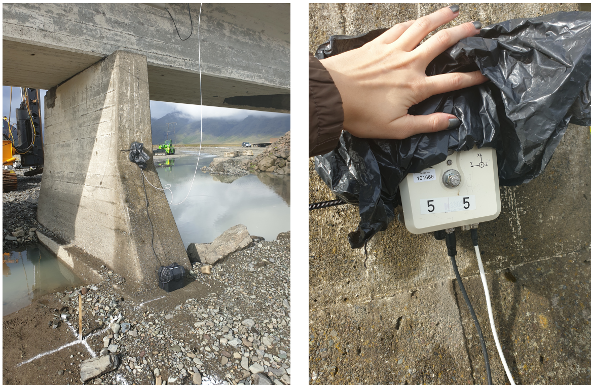
Figure 2.10: The placement of the accelerometers on the pillars.
