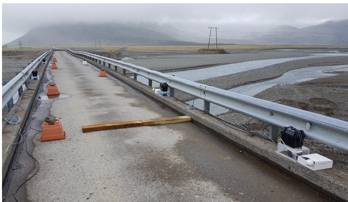
Figure 2.1: Accelerometers from ETH and RU distributed along the deck of the bridge.
