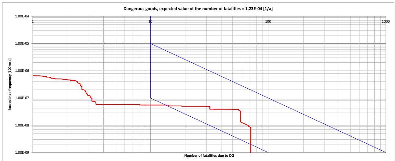
Figure 6.15 FN-curve for dangerous goods accidents. Fatalities per 100 m section per year, northbound, 2033.
